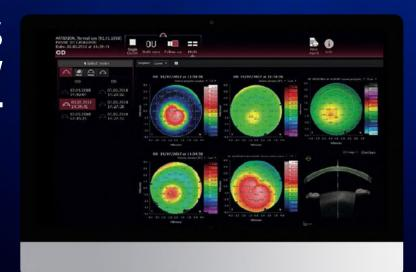
The combination of total corneal power, pachymetry and corneal wavefront analysis delivers the detailed information required for confident decision making.
